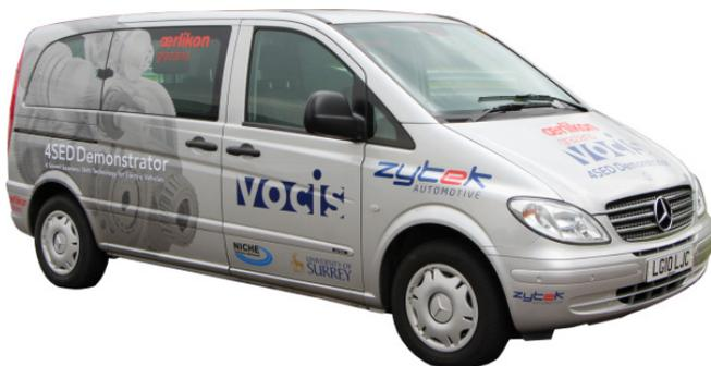
Mercedes Vito Minibus: Fully electric demonstrator vehicle from Oerlikon Graziano and Vocis equipped with the power shifting 4SED transmission
